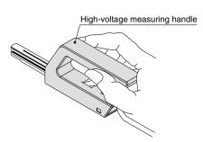
Note) Be sure to use a high-voltage measuring handle in situations such as during highvoltage measurement when there is a possibility of personnel coming in contact with electricity.
